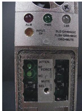
Figure #4: MAXNET II MPTX8 Front Panel Pushbuttons
