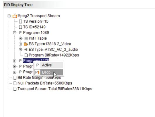
To reactivate a dropped program, right-click the program in the PID Display Tree and select **Active** from the drop-down list. The program is returned to the processed stream and removed from the Add & Drop Settings box.
