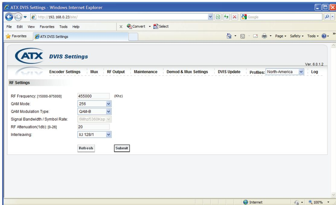
The RF frequency output range is 15 to 975 MHz, entered in kHz without decimal points or commas. In the example above, a setting of 455 MHz is entered as 455000.
