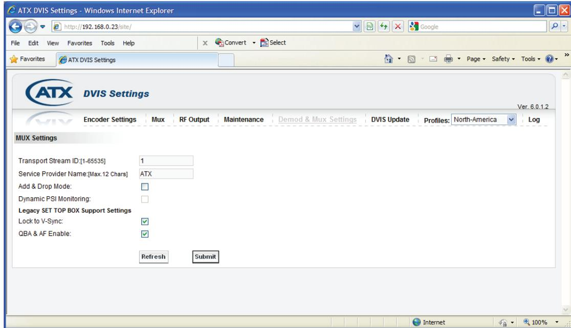
When Add/Drop is enabled, certain parameters in the DVISm GUI screens are not accessible; these fields are greyed out and inaccessible (Section 1.7, Demod & Mux Settings, shows which parameters are settable and which are locked).
