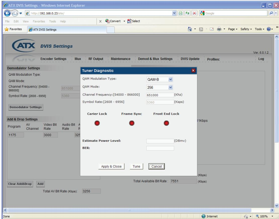
2. Select the QAM Modulation type and QAM mode. Enter the Center Frequency of the desired QAM channel (kHz).
