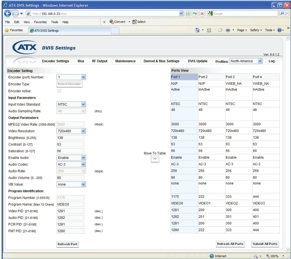
Similarly, the Mux menu shows the status of Add & Drop Mode, Dynamic PSI monitoring, etc.; the RF Output menu shows output frequency, QAM Mode, etc.; and the Maintenance menu shows the status of the DVIS unit. Parameters that can not be changed are greyed out.
