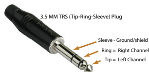
Figure 6-2: 3.5 MM TRS Connections
