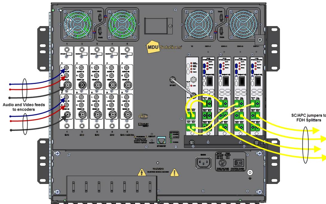
Figure 3-6: Panel Connections
