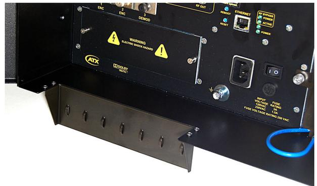
Figure 3-10: Cable Management Bar Inverted Outward
