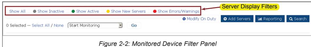
Figure 2-2: Monitored Device Filter Panel
