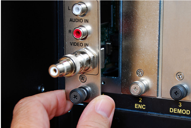
Release Screw and Gently Pull Card Out
