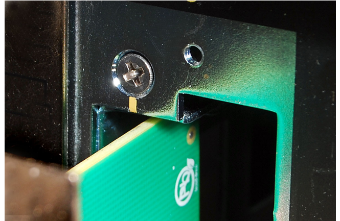
To Replace - Align Card with Yellow Card Slot Marker
