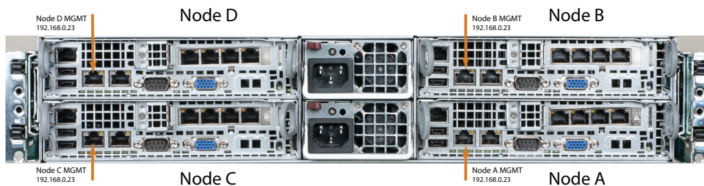
Figure 3-1: Rear Panel MGMT Ports - Identical IP Addresses
