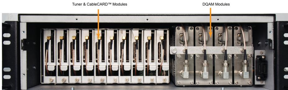
Figure 2-3: Version 2 QAM to QAM Front Inside
